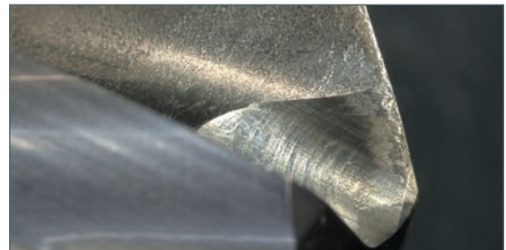
Tool cutting edge before decoating process
